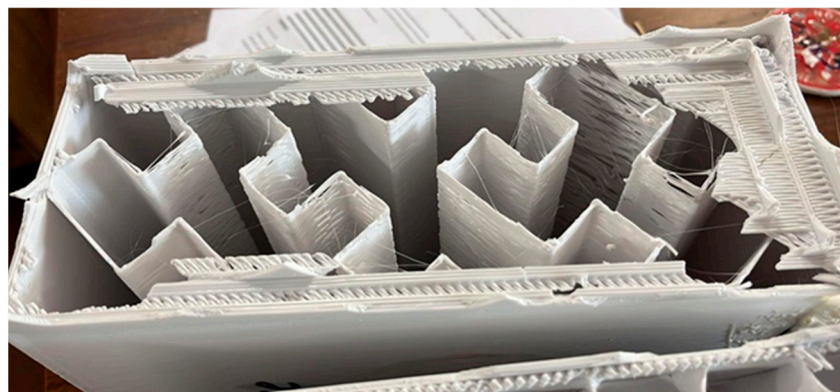
Figure 11. Cross-section of the Hilbert curve specimen with 5% infill density.
