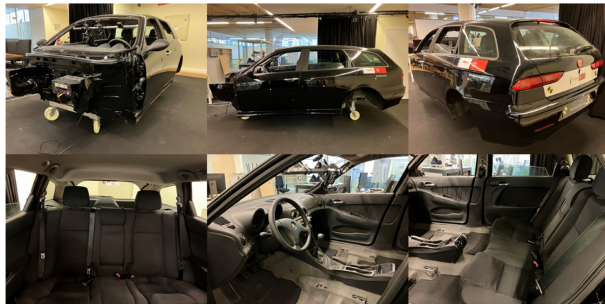
Figure 5. Laboratory car testbed from different perspectives.
