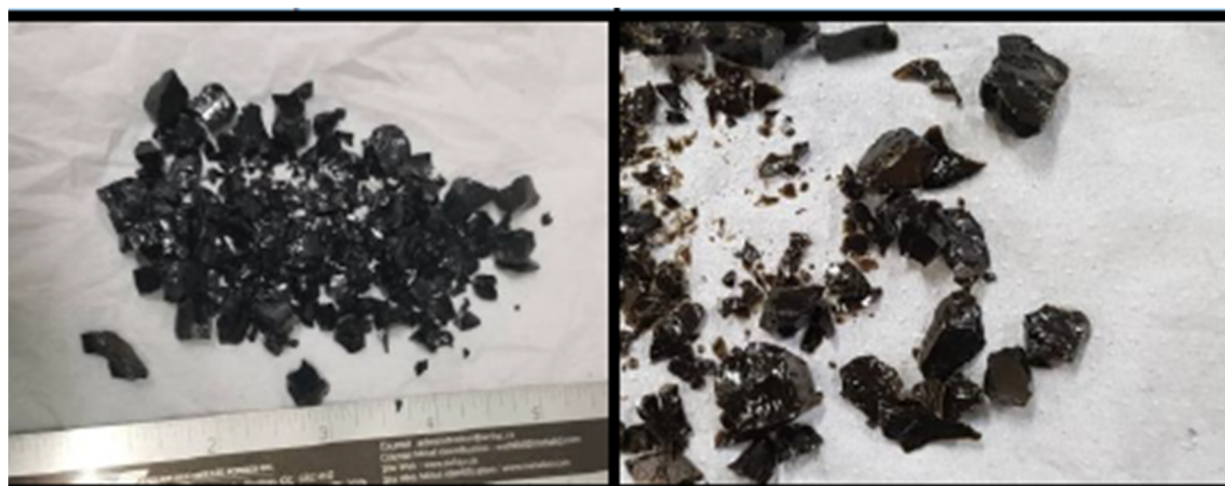
Figure 7. Glass formed from GlassRock™ methodology demonstrates the possibility of As and Sb recovery and its use as an industrial product.
