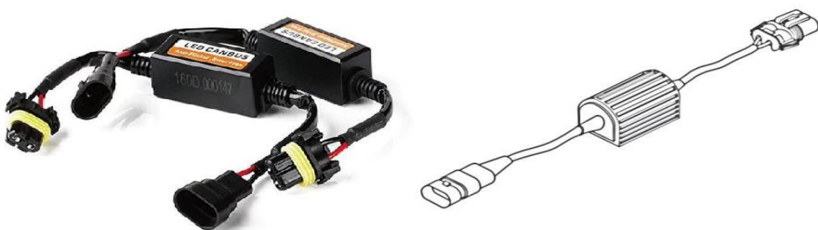
Figure 7 - Example of CAN Bus Harness (Petrescu et al. , 2019)
