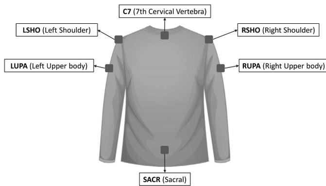
Fig. 1. IMUs position within the ergonomic vest.
