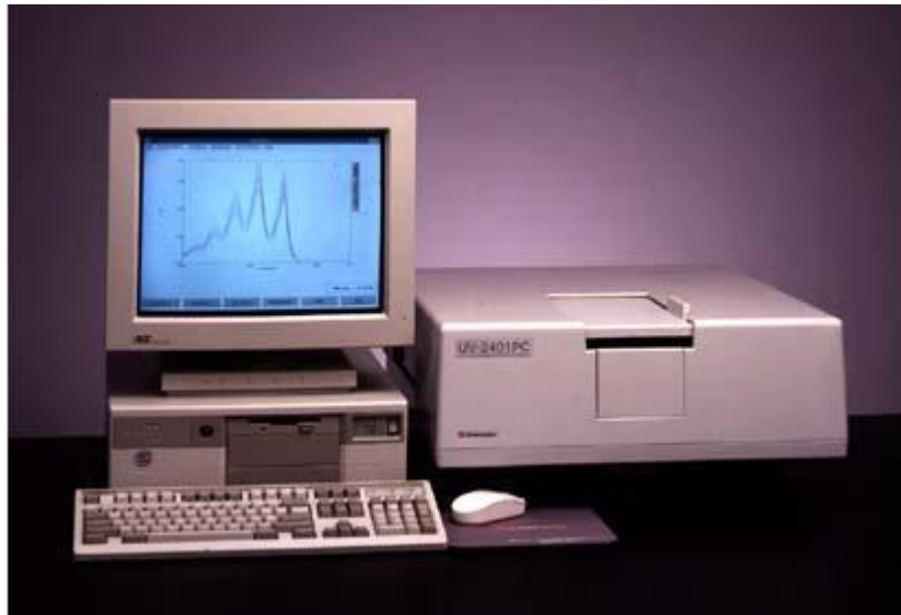
Figure 4: Shimadzu UV-2501PC UV-Vis spectrophotometer for transmittance and reflectance measurements in the Vis/UV range.
