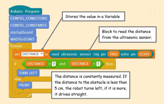
Don't forget that for the program to work, you still need to write the TURN LEFT and FRONT procedures.
