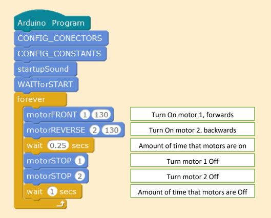
NOTE: Take a sheet of A4 format and test whether the robot turns correctly. If the turn is too small, increase the turning time or speed.
