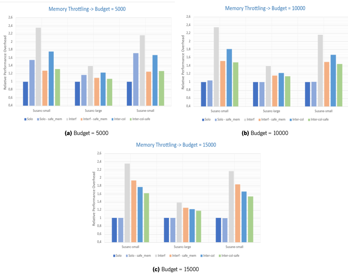
Figure 4.9: Performance Overheads of Mibench automotive benchmark for different budget values relative to a Linux guest Execution, analyzing the collaboration between the mechanism implemented and the existing cache coloring mechanism.
