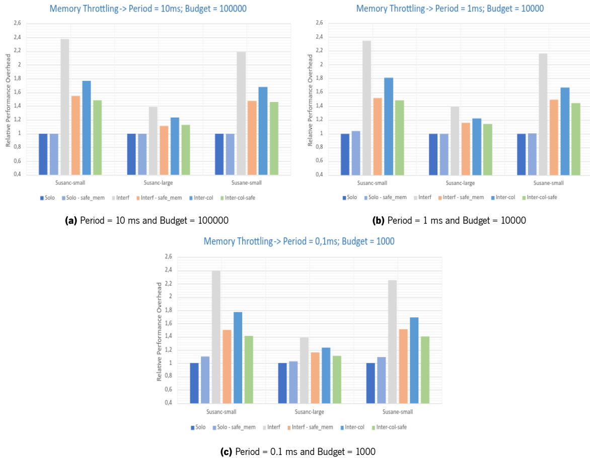
Figure 4.10: Performance Overheads of Mibench automotive benchmark for different budget values relative to a Linux guest Execution, analyzing the collaboration between the mechanism implemented and the existing cache coloring mechanism in three different periods.
