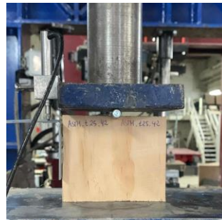
Figure 3: Test setup within ASTM D 5764-97a [5]
