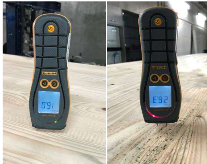
Figure 2: Measurements of the surface moisture content of wood using the electrical resistance method.
