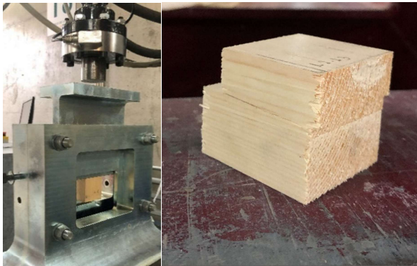
Figure 3.2: Shear tests parallel to the grain performed on small specimens
