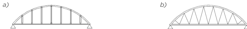
Figure 9.23 W Hanger systems, adapted from (Han, et al., 2016) a) Langer and b) Nielsen
