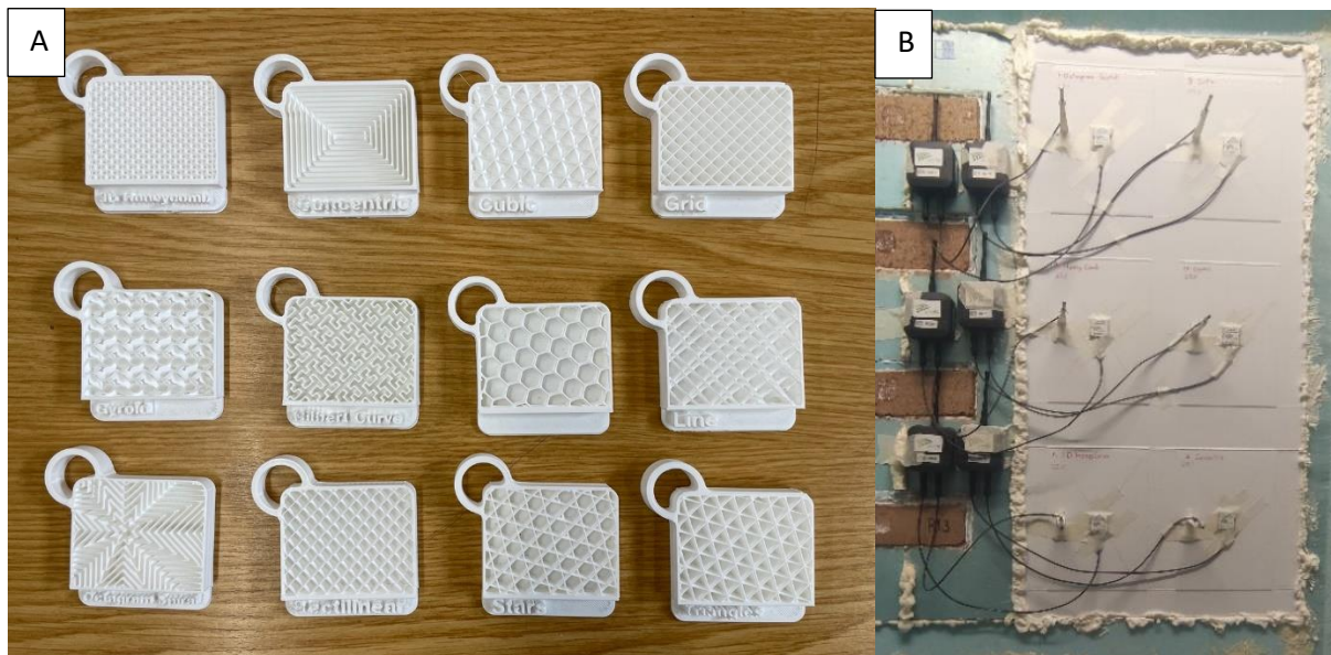
Figure 4. Left-A illustrates the twelve infill patterns chosen to estimate their influence on thermal performance. The right-B represents the hotbox proceeding to calculate the thermal conductivity of the panel, each one with six samples. Six heat flux sensors were installed in the centre of each sample. The authors took both photos during the laboratory test.
