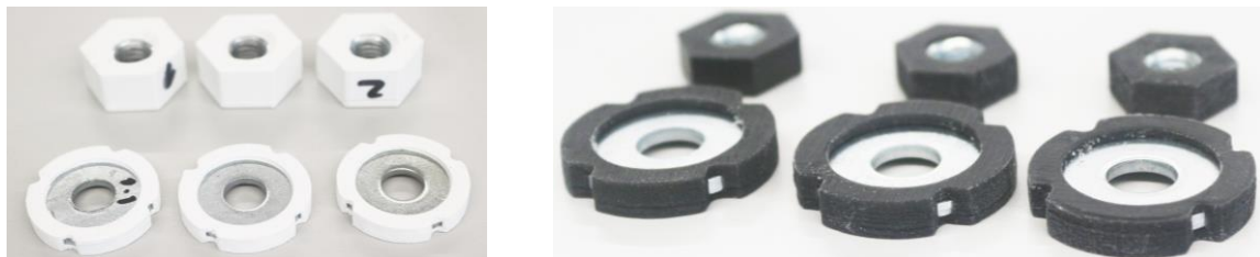
Figure 9: Resulting prototypes for: (a) FDM process; and (b) Polyjet process.
