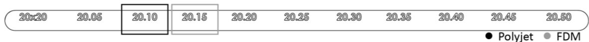
Figure 6: Representation of the ruler and the most suitable result for each technology.
