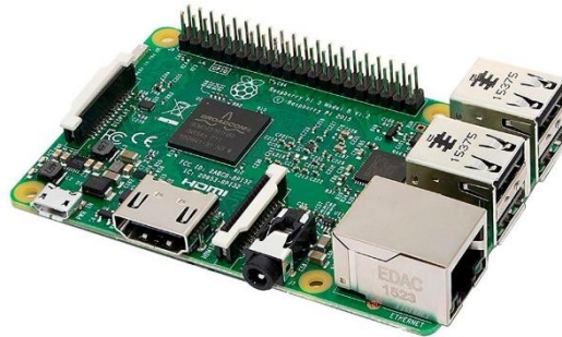
Figura 10 - Raspberry Pi 3B+ [34]
