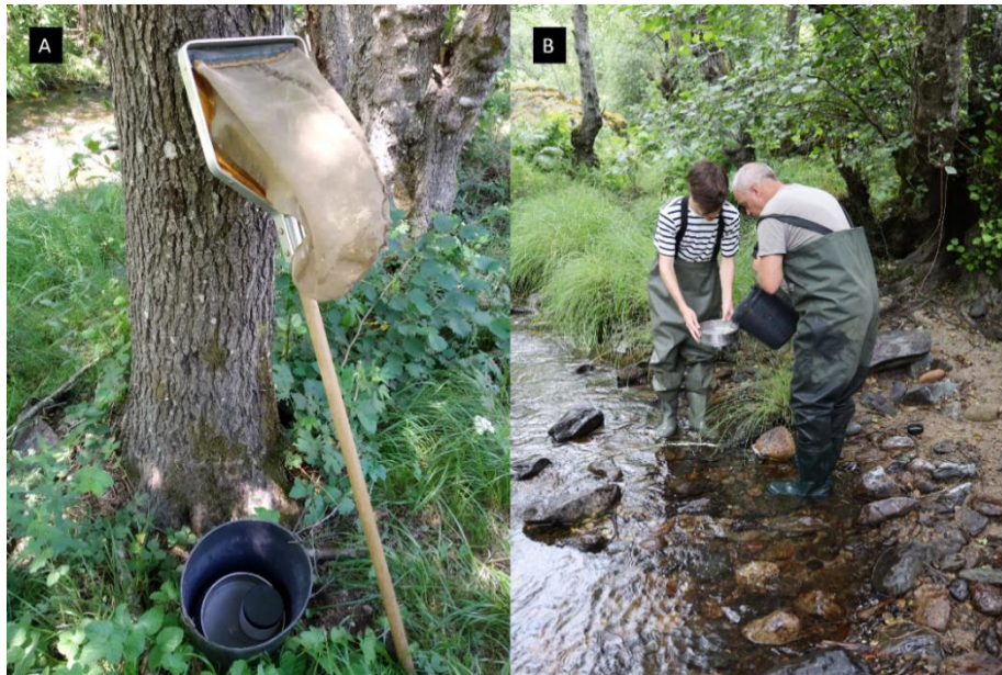
Figure 4 - A - Material used to collect macroinvertebrates (hand net, sieve, bucket, and jar). B - Sampling process, which involves passing the sample collected with the hand net through a sieve.
