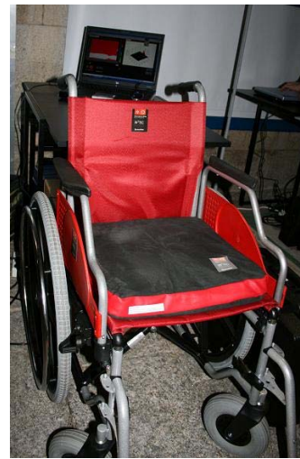
Fig. 12. First prototype – Cushion for wheelchair with sensor matrix and monitoring system.
