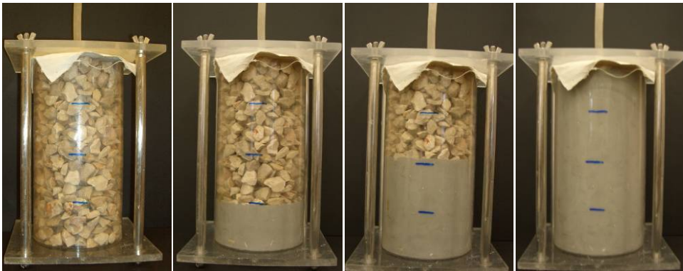
Figure 4 – Example of filling cylindrical molds (product D and limestone)
