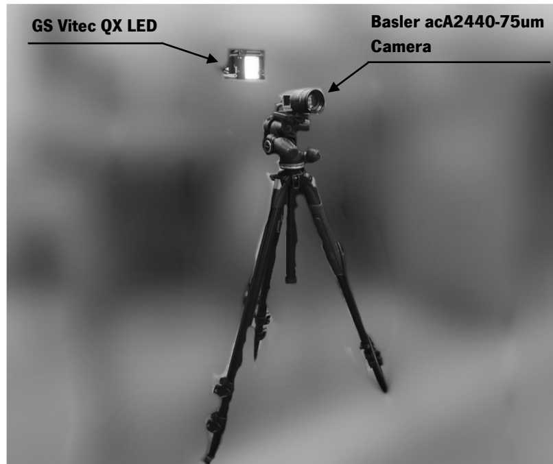
Figure 8.5 – Illumination LED and camera utilized for the slider's tracking procedure.
