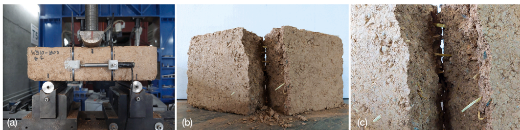
Fig. 8. Three-point bending test on a WS10 block.
