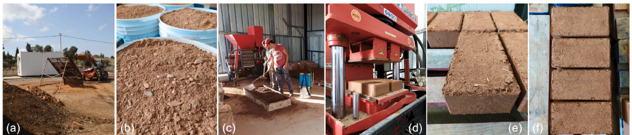
Fig. 2. Main steps of the production process of the CEBs involved in this study.
