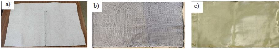
Fig. 2. Materials used to produce the structures. a) Recycled polyester nonwoven; b) Basalt fibre fabric; c) Aramid fibre fabric.
