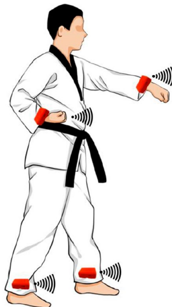
Figure 5. Positioning of motion sensors on a Taekwondo athlete's wrists and ankles.
