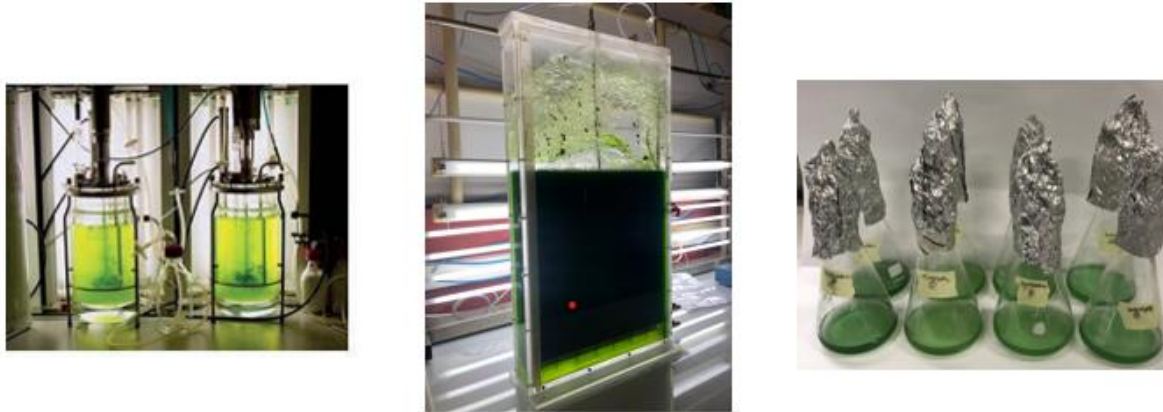
Figure 5. Examples of lab-scale production of microalgae: mechanically agitated reactors, flat panel photobioreactors, and Erlenmeyer flasks. Based on Enzing et al., (2014).
