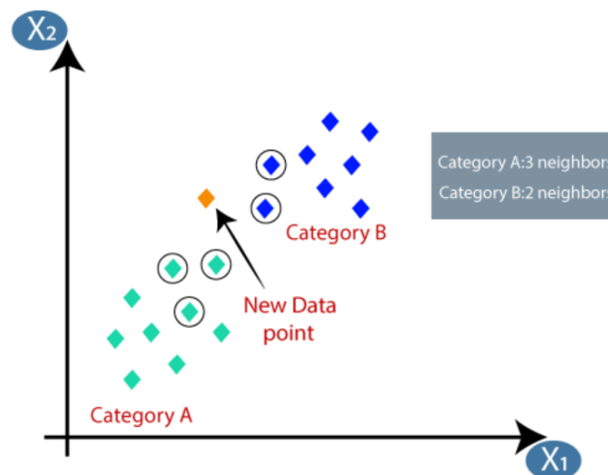
Figure 21 - Results of a KNN Algorithm, retrieved from ( https://www.javatpoint.com/k-nearest-neighbor-algorithm-for-machine-learning )
