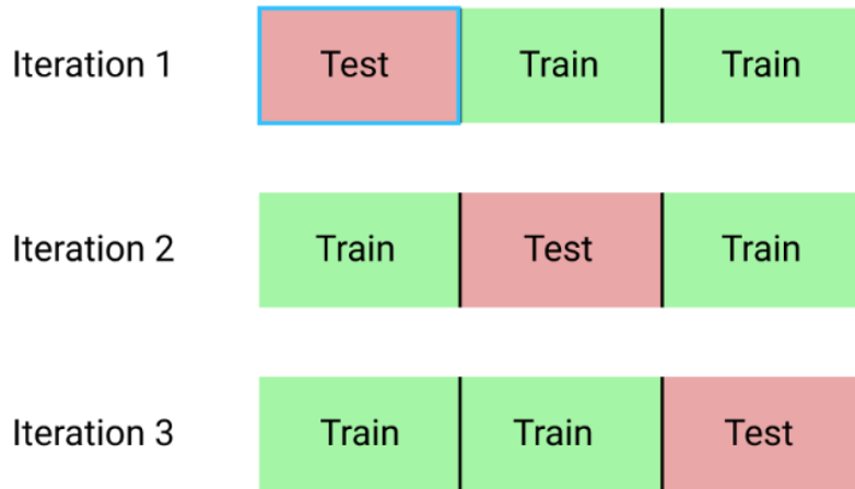
Figure 14 - Example of K-Fold Cross-Validation
