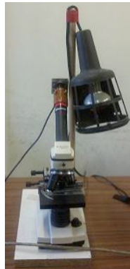
Fig. 7. Yarn image capture system [14]
