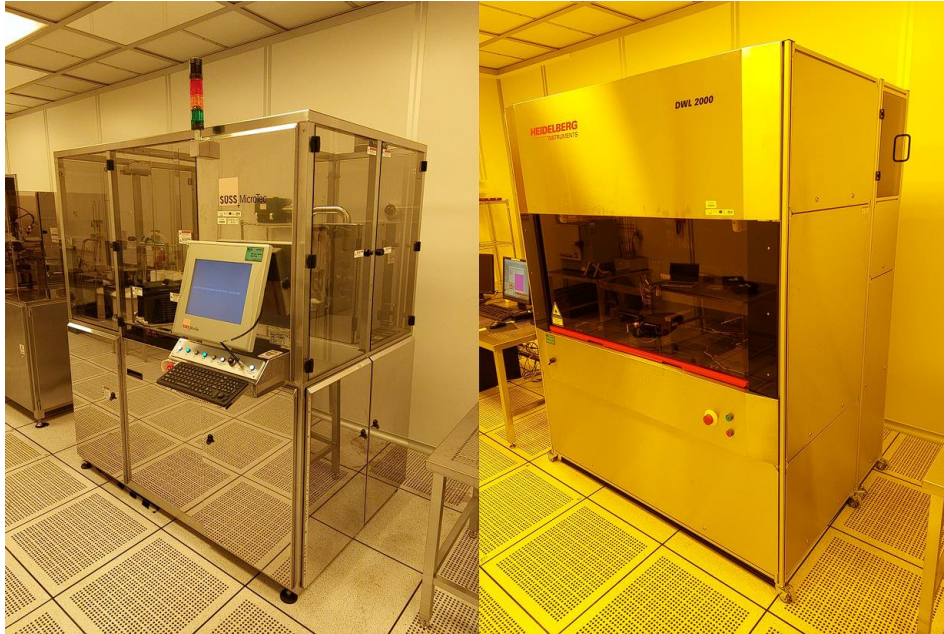
Figure 24 – Systems utilized in photolithographic processes. (Left) Utilized SUSS Microtec Gamma Cluster system for spin-coating of photoresists of different thicknesses, (Right) Utilized Heidelberg DWL 2000 system for lithography patterning of the photoresist.
