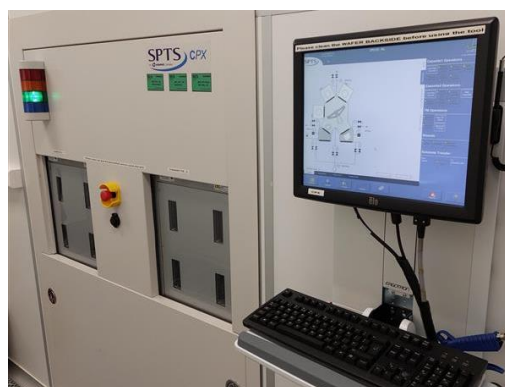
Figure 22 – Utilized SPTS CVD MPX system.
