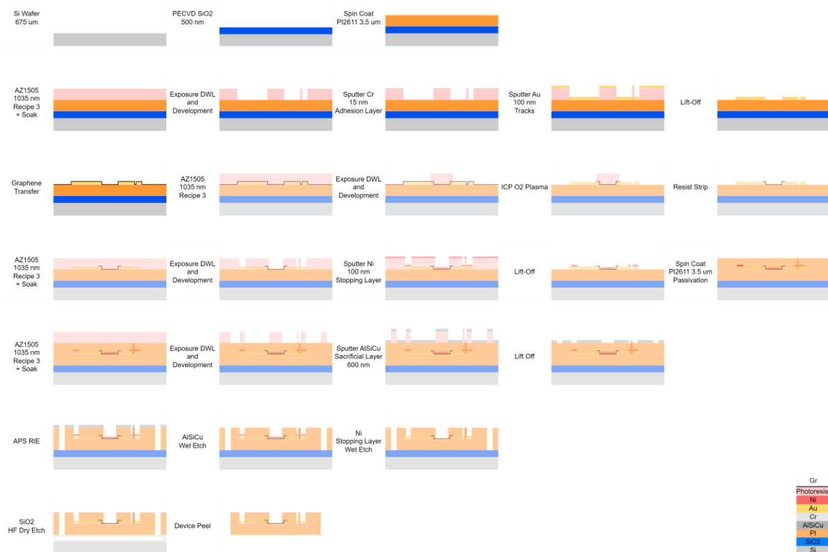
Figure 78 - Schematic of the fabrication steps of the device wafer. The non-executed fabrication steps are represented in fainter colors.
