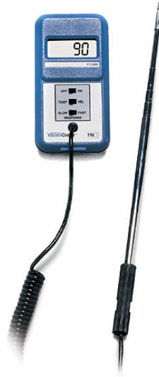
Figure 3.7: Thermo-anemometer model 8330 from TSI VelociCheck.
