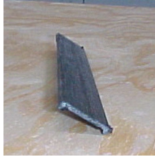
Fig. 9. U-Shape GF/PP pultruded profile made from towpregs
