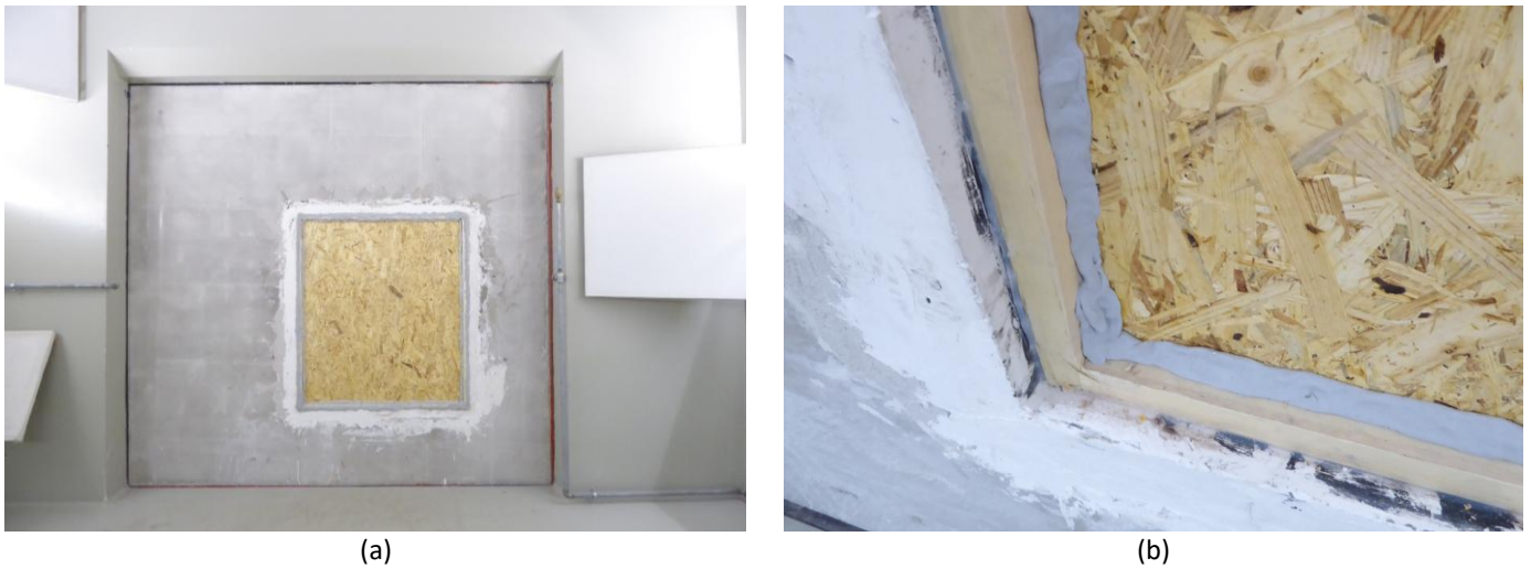
Figure 2. Illustration of a tested wall panel: (a) view from the source chamber; (b) panel sealing detail.
