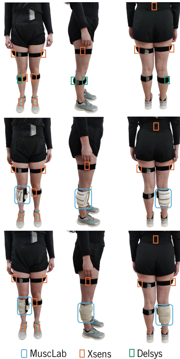
Figure 4.5 – A participant instrumented with the (i) Trigno Avanti and Xsens Awinda systems (top view); (ii) Trigno Avanti, Xsens Awinda, and MuscLab (without outer band) systems (middle view); and (iii) Trigno Avanti, Xsens Awinda, and MuscLab (with outer band) systems (bottom view).
