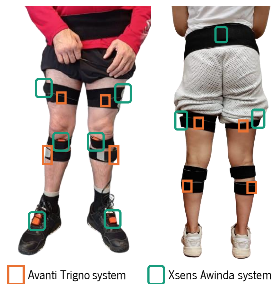
Figure 7.4 – Post-stroke patients instrumented with the Trigno Avanti and Xsens Awinda systems.
