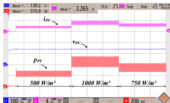
Fig. 13. Current, voltage, and power of the PV array.
