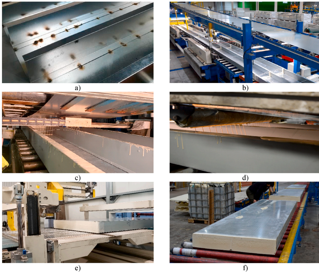
Fig. 3. Example of the manufacturing process of the prototype sandwich panel: a) placement of vertical elements (webs); b) bottom and top face sheet on production line; c) adhesive on top of web and uncoil of upper face sheet; d) injection of the liquid PUR compound that forms the foam; e) placement of panel in packaging line for cutting/trimming; f) final aspect of the manufactured panel.
