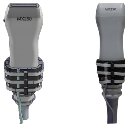
Figure 45: Sensor holder design in SolidWorks (left) and its real 3D-printed implementation attached to the MX250 probe (right).
