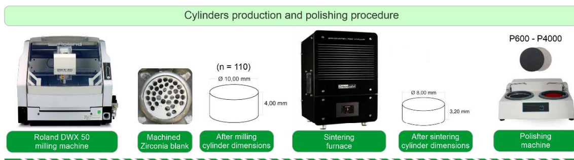
Figure 4.1 - Sequential depiction of the 3Y-TZP zirconia cylinders' production process, encompassing machining from a pre-sintered block, sintering under specified conditions, and subsequent polishing to achieve a smooth finish.
