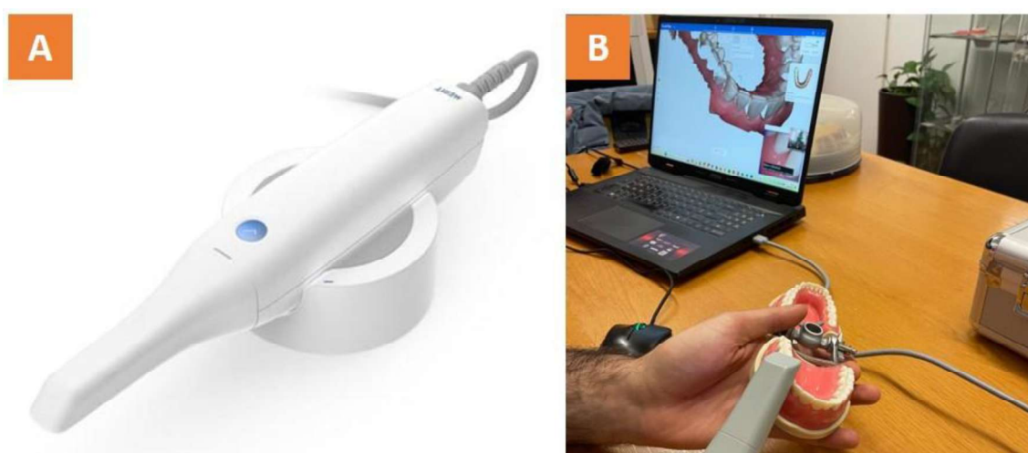
Figure 6.2 - Medit i500 intraoral scanner (A) and scanning process (B).
