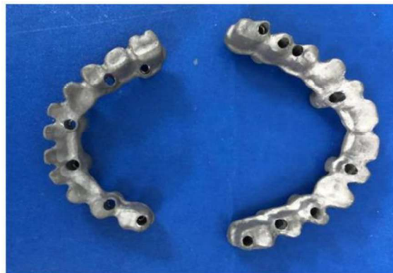
Figure 2.10 - Cobalt-Chromium alloy frameworks [50]
