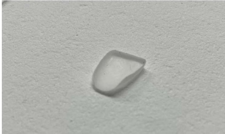
Figure 6.12 - Final appearance of the veneer after sintering
