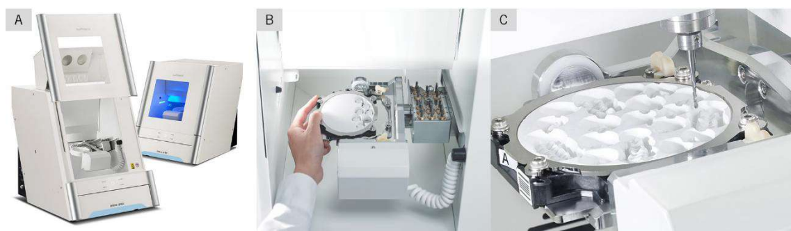
Figure 2.14 - DWX 51D five-axis milling unit by Roland DG. (A) Overview of the equipment used for milling ceramic restorations. (B) Detail of the zirconia disc fixation process within the milling unit. (C) Close-up of the simultaneous milling of multiple structures in the zirconia block. [Adapted from Roland DG, Japan].
