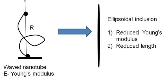
Figure 4.11: Substitution of curved nanotube with ellipsoidal inclusion
