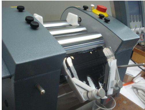
Figure 2.6: Calendaring (or three roll mill) machine used for particle dispersion in a polymer matrix (Polymer Department, University of Minho)
