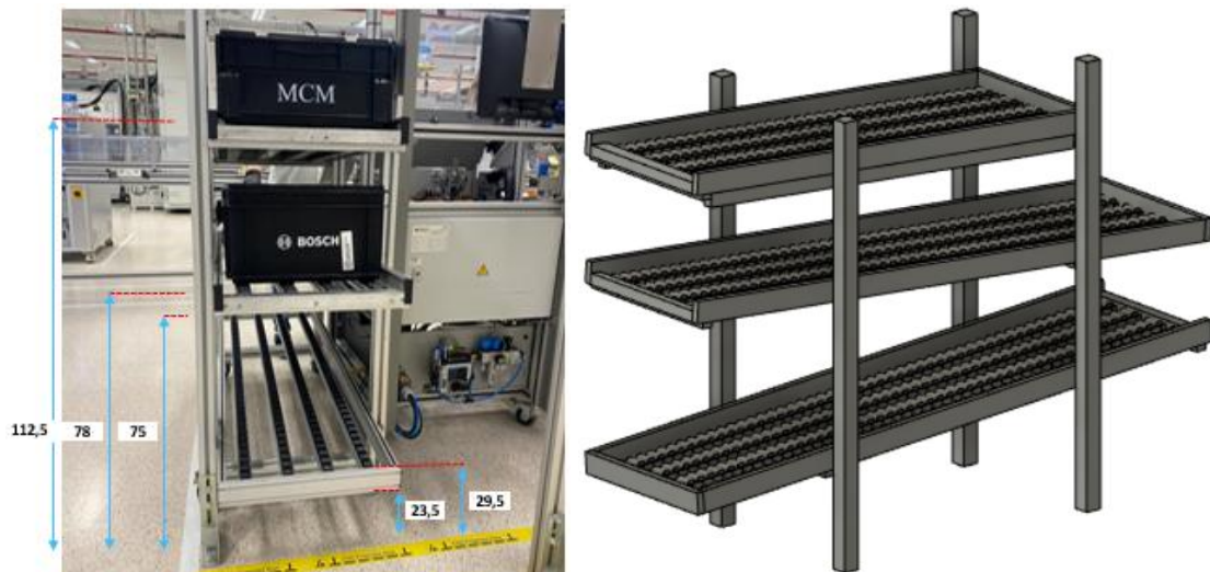
Figure 39 - Two-level access ramp for the storage of Targets .
