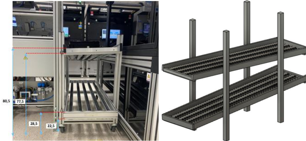
Figure 38 - One-level access ramp for the storage of Targets .
