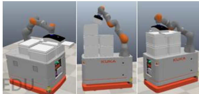
Figure 57 - Study of the maximum number of 400x300 boxes on the platform.
