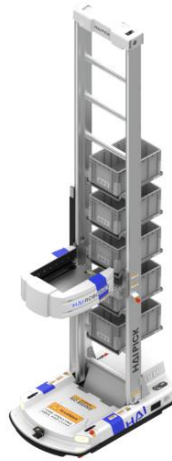
Figure 6 - Autonomous Case-handling Robotic System (ACR) from HAI ROBOTICS. Adapted from (H. Robotics, 2022).
