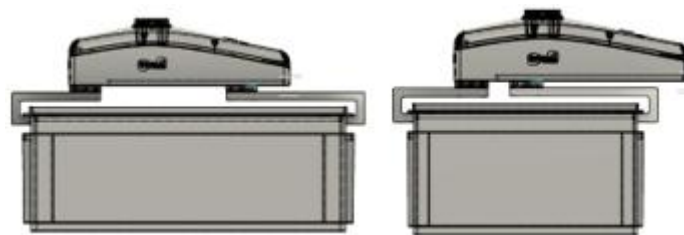
Figure 47 - Gripper holding the two types of Targets .
