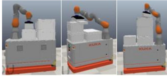
Figure 58 - Study of the maximum number of boxes of both types on the platform.
