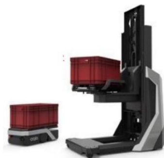
Figure 7 - Skyler and Cart robots from Caja Robotics. Adapted from (C. Robotics, 2023).
