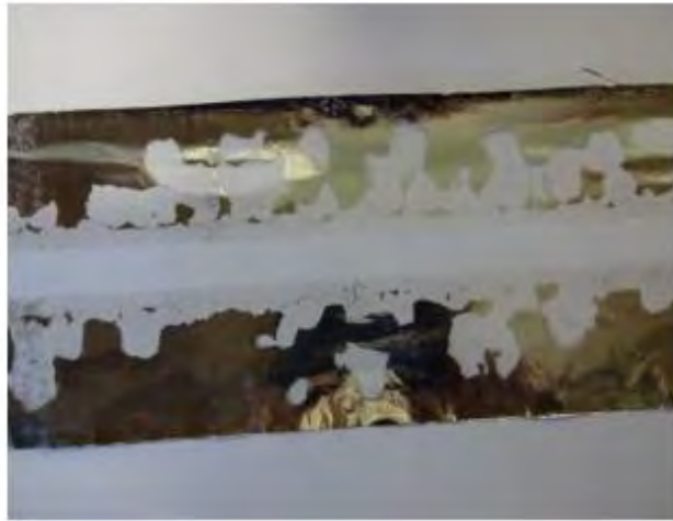
Figure 8- Metallized film which was demetallized due to corona arcing [14]
