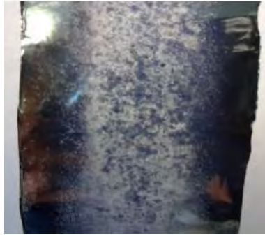
Figure 7- Metallized film with electrode corrosion due to the presence of moisture [14]
