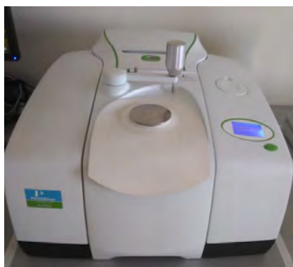
Figure 32- PerkinElmer ATR-FTIR, model Frontier
