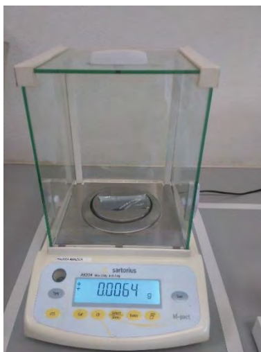
Figure 31- Weight of a BOPP sample
