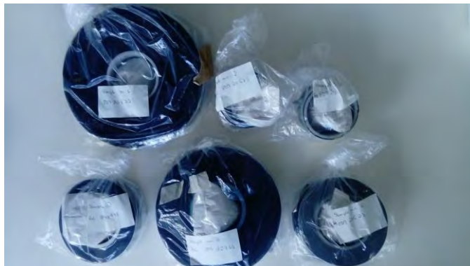
Figure 29- Metallized polypropylene film samples
