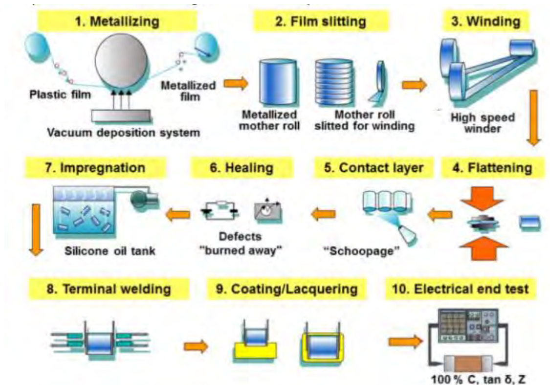
Figure 4- Steps for a film capacitor manufacturing [10]
