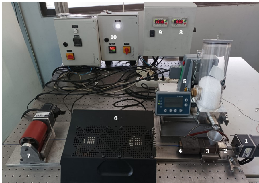
Figure 3.1: Microextrusion Line: 1 - DC Motor, 2 - Transmission system, 3 - Barrel, 4 - Die, 5 - Volumetric feeder, 6 - Cooling fans, 7 - Haul-off, 8 - Haul-off speed controller, 9 - Screw speed controller, 10 - Temperature controller.
