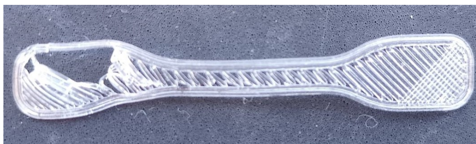
Figure 5.37: On the left: Failed attempt to print at 190 °C. On the right: Some of the printed test specimens.
