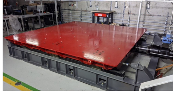
Fig. 3: 1D shake table of the University of Minho
