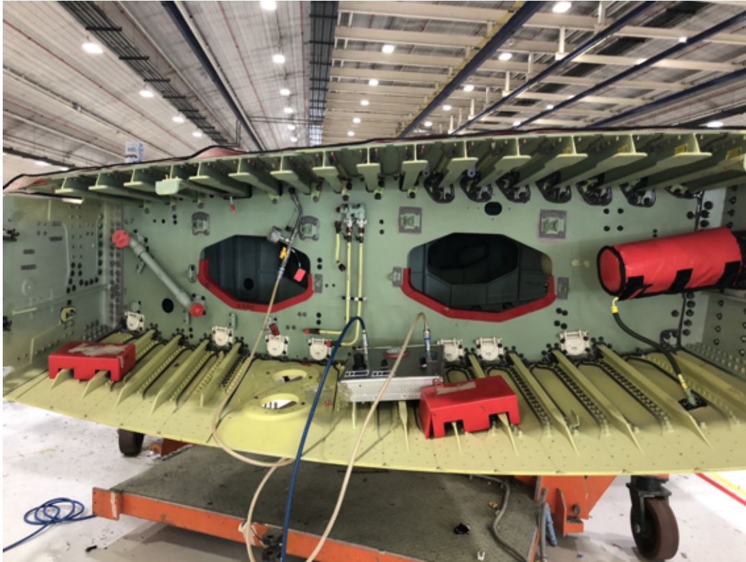
Figure 7: Interior of an integral wing fuel tank.
