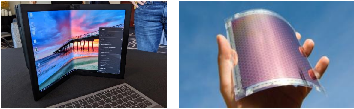
Figure 1.1. (a) Foldable OLED display (reprinted from [9]). (b) Organic photovoltaic cells (reprinted from [10]).
