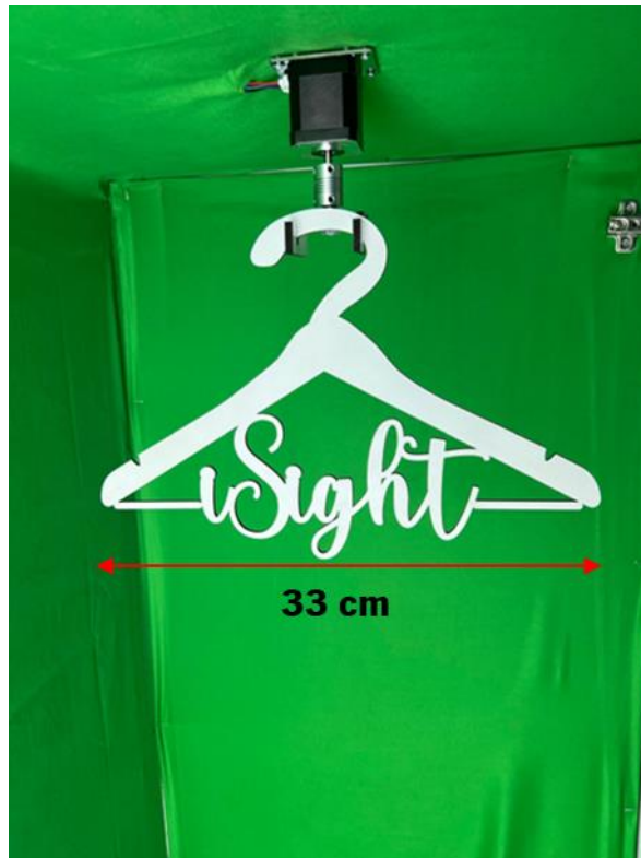
Figure 5.17: Motor supporting the hanger.
