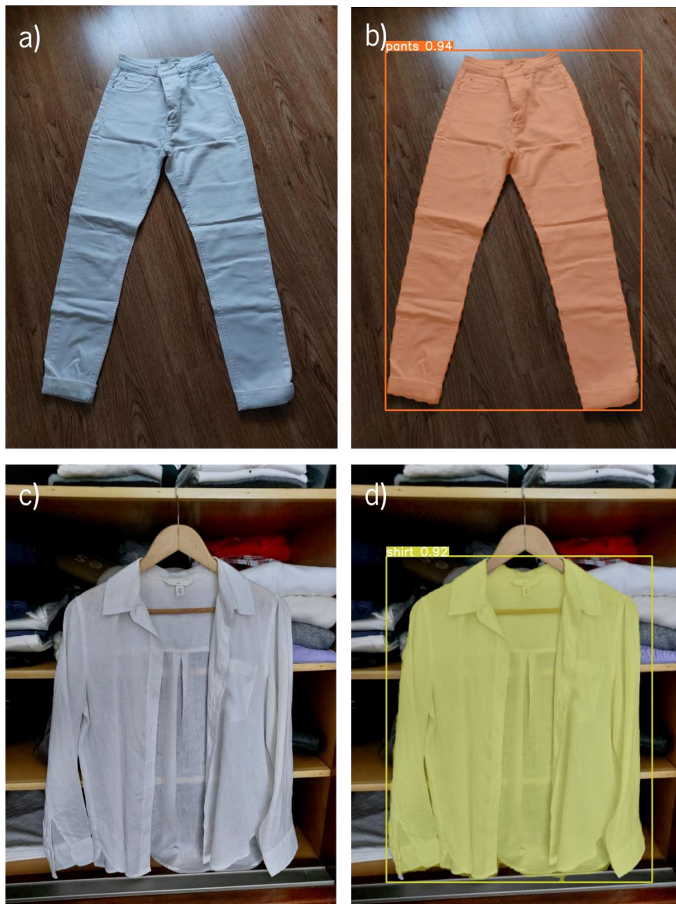
Figure 4.11: Example of inference images with category and respective segmentation mask: (a) Original image of pants; (b) Segmented image of pants; (c) Original image of a shirt; (d) Segmented image of the shirt.
