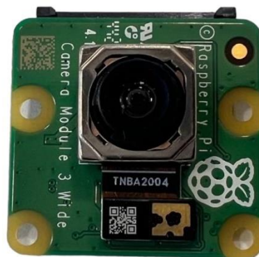
Figure 5.6: V3 Oficial Raspberry Pi, 12MP, 120°, camera module, used in the developed prototype.
