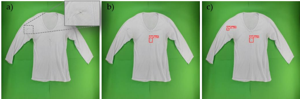
Figure 4.19: Example of a defect undetected by the YOLOv5m6 model that was subsequently identified with the aid of data augmentation: a) original image; b) predicted image from model YOLOv5m6 without augmentation; c) Predicted image from model YOLOv5m6 with augmentation (Rocha, Pinto, et al. , 2023).
