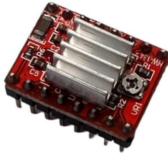
Figure 5.4: Picture of the driver motor A4988 used in the developed prototype.
