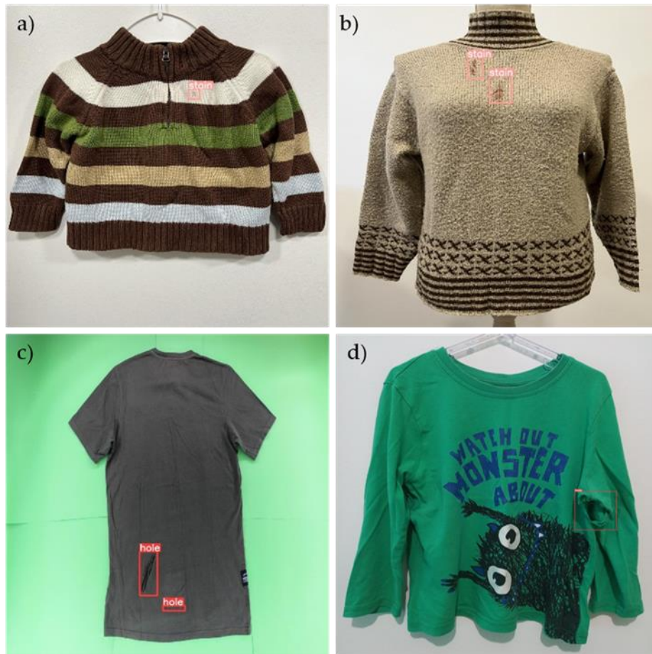
Figure 4.21: Examples of predicted images from the YOLOv5l6: a) single stain detection; b) multiple stain detection; c) multiple hole detection; d) hole detection near the seam (Rocha, Pinto, et al. , 2023).
