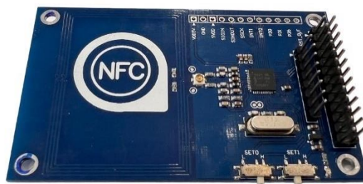
Figure 5.7. ITEAD PN532 NFC reader used in the developed prototype.
