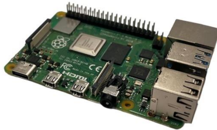
Figure 5.5: Picture of a Raspberry Pi 4 Model B used in the developed prototype.
