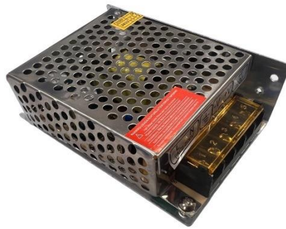
Figure 5.9. Picture of the 12V 60W 5A power supply incorporated in the developed prototype.
