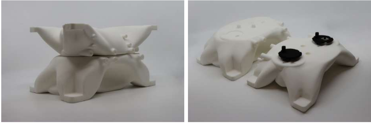
Figure 38: Prototype of the moulding tool
