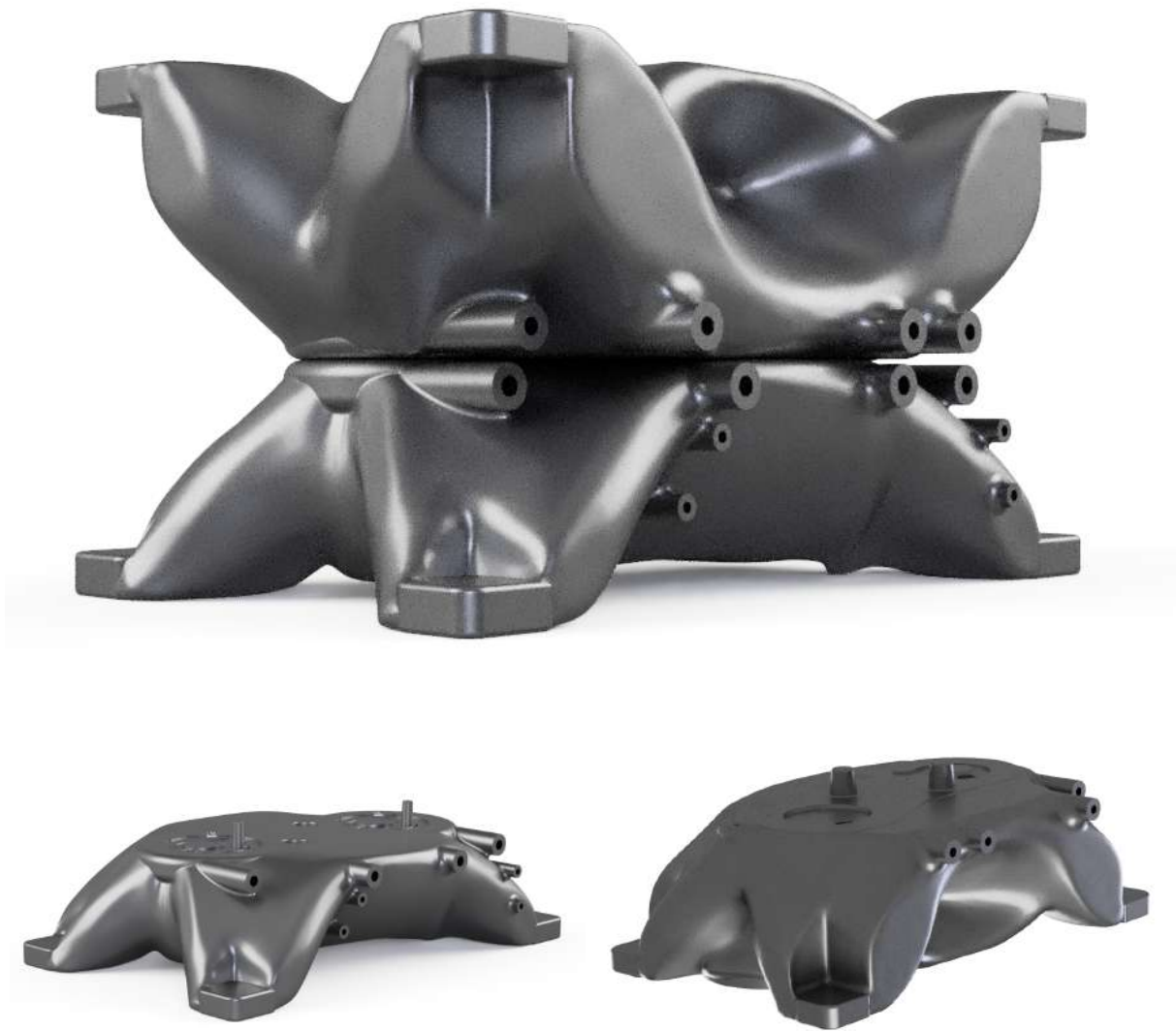
Figure 39: Final model of the moulding tool
