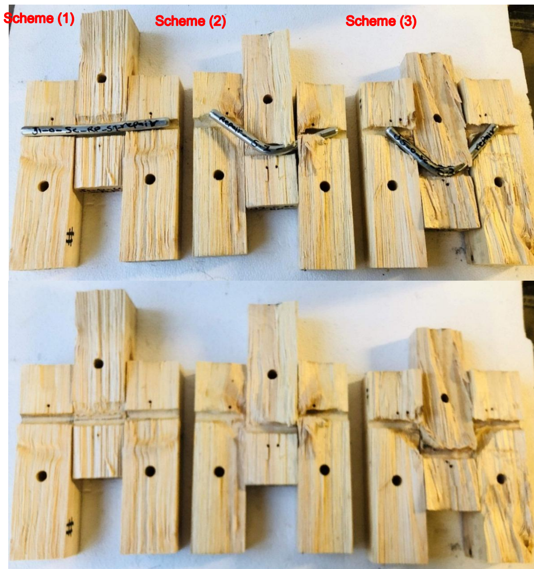
Figure 3:55 - Failures associated with scheme (1), (2) and (3) for joints with 12 mm dowels.
