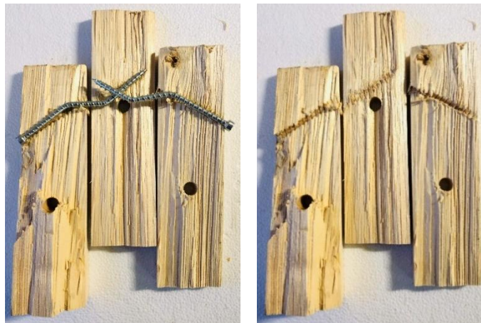
Figure 3:53 - Top: Dowel deformation, Bottom: Screws' deformation
