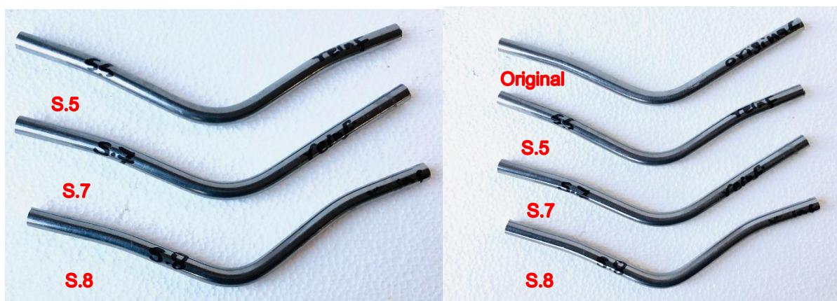
Figure 3:34: Left: failures in the dowels of the 3 schemes, Right: failures in comparison to the original joint
