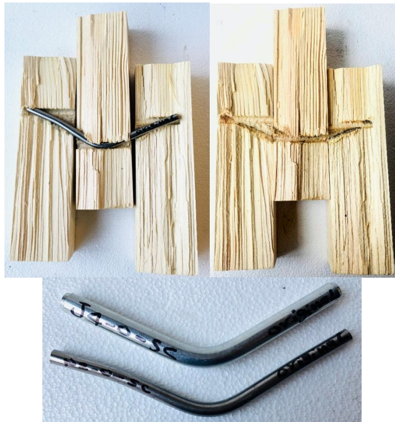
Figure 3.12: Top left: New joint after testing with 8 mm dowel, Top right: dowel embedment into surrounding fibres, Bottom: 12mm and 8mm dowels after testing
