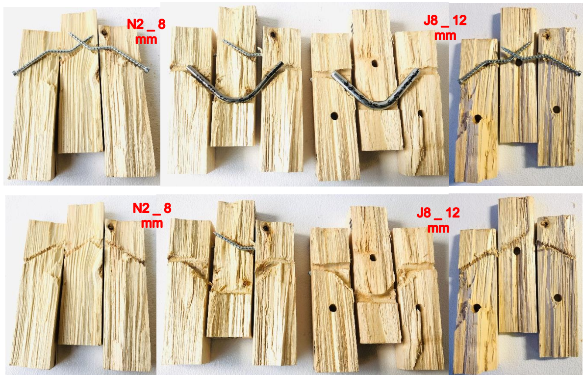
Figure 3:57 - Left: Failure on 8 mm dowel joint, Right: Failure on 12 mm dowel joint.
