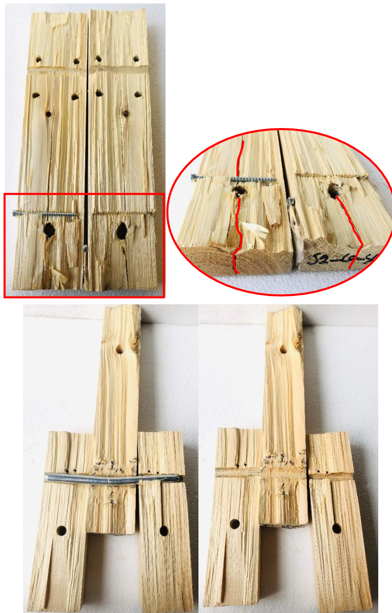
Figure 4:13 - Left: Dowel's deformation, Right: Screw deformation.
