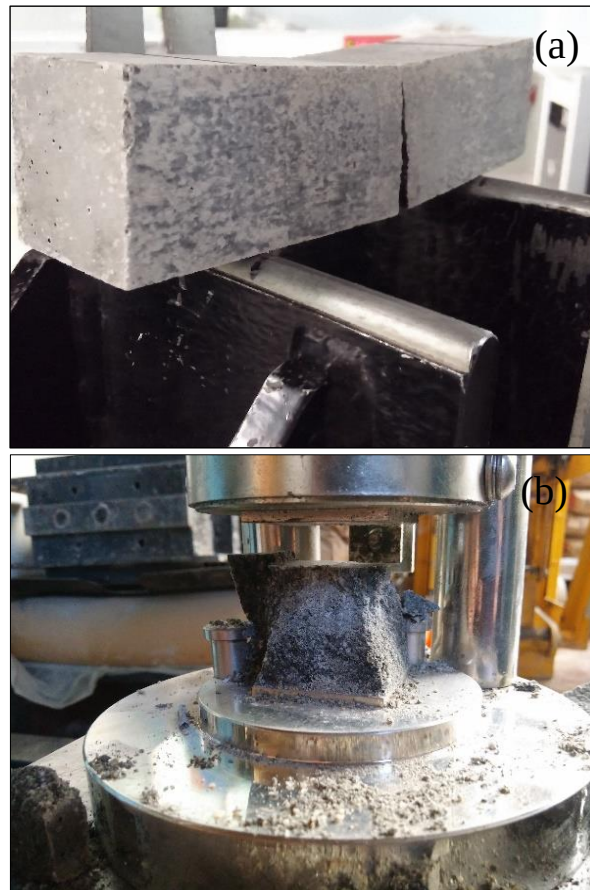
Figure 4-10: Images of specimens after tests: a) specimen GC(0.5%) after flexural test, b) specimen GC(0.5%) after compression test.
