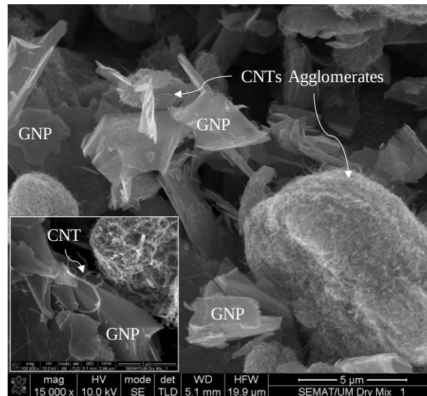
Figure 4-1: Morphology of CNTs and GNPs dry mix.
