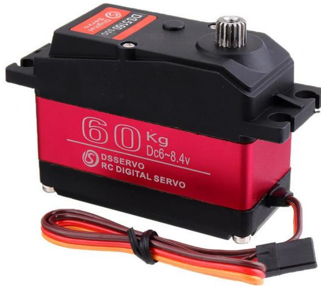
Figure 26 - João Martins, 2022 - Mechanical Arms Feet Platform – Servos.
