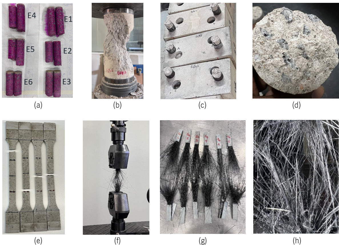
Figure III.8. (a) Carbonation of concrete; typical failure modes from: (b) concrete under compression; (c,d) concrete under tension (pull-off tests); (e) epoxy adhesive under tension; and (f to h) CFRP laminate under tension.
