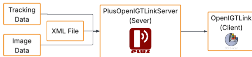
Figure 6.7: Workflow linking the data acquisition, the PLUS server, and the 3D Slicer client through the OpenIGTLink protocol.
