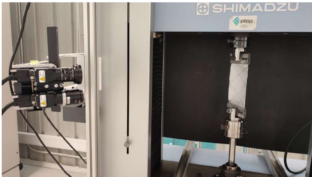
Figure 4.8: Bias extension test: experimental setup.
