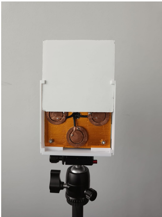
Figure 26: Real assembly. Left: module mounted with sliding cover in place. Right: Female screw for tripod
